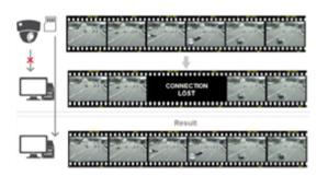
In the event of intentional or accidental damage to the recording server, ACTi cameras can record evidence directly to SD cards. Once the server is back online, the camera can transmit the recorded data to the NVR, ensuring no loss of evidence.
