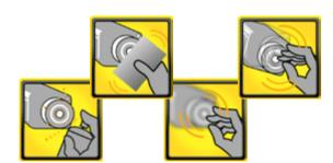
Camera manipulations such as covering the lens or redirection can be detected and a notification can be immediately sent to the control center.
