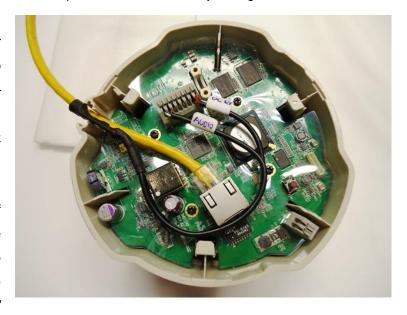
whereas the two wires of power supply are connected to the pins "DIO PW" and "DIO"GND" of the terminal block. Please note that the power circuit connected this way will work continuously regardless of the DI and DO levels.
