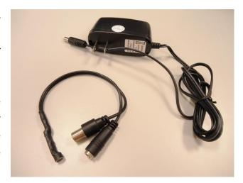
However, if your intention is to build a pure PoE-based camera solution, then you would not want to hassle with additional power supply just because of the microphone. With ACTi DI/DO supported cameras it is possible to use the power supply of DI/DO system of the camera to feed the active microphone! Most of ACTi DI/DO systems in the camera provide DC 12V power, therefore please keep that in mind while choosing the active microphone – make sure it is working with DC 12V power supply.
