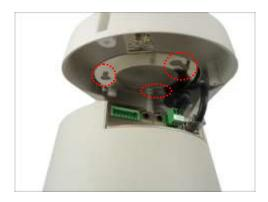
3. Slide the camera clockwise to secure the hooks to the mount.
