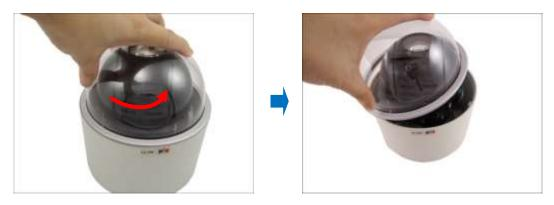
2. Rotate the replacement dome cover clockwise to attach it.
