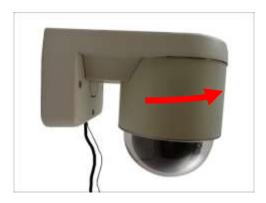
4. Attach three (3) screws (included in the L-type wall mount package) to secure the camera to the mount.
