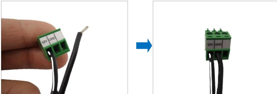
4. Tighten the screws of the **12V** pin and the **GND** pins to secure the wire connection.
