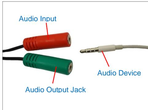
If the camera is installed outdoors, be sure to wrap the audio connectors with Waterproof tape (can be purchased in hardware stores).
