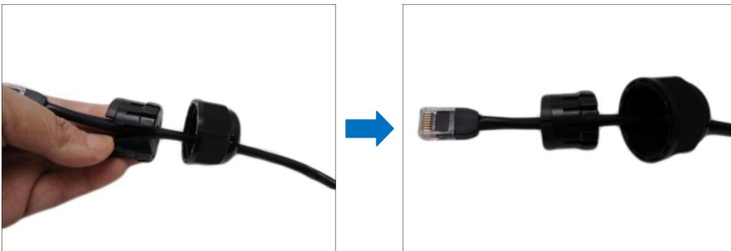
4. Attach one (1) supplied rubber ring on the gland body (smooth end).
