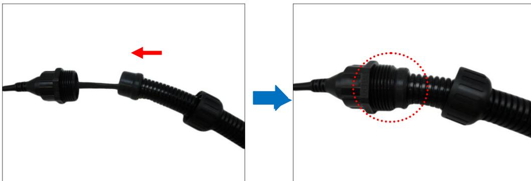
9. Attach the clamping nut to the conduit gland body. Make sure the clamping nut is tightly secured to avoid water leakage.
