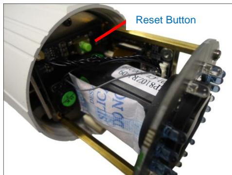
**NOTE:** DO NOT remove the desiccant bag inside the camera to keep the interior parts dry.
