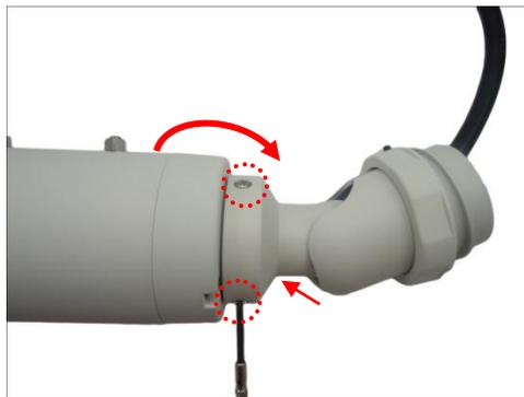
3. Attach the three (3) screws to attach the integrated bracket to the camera.
