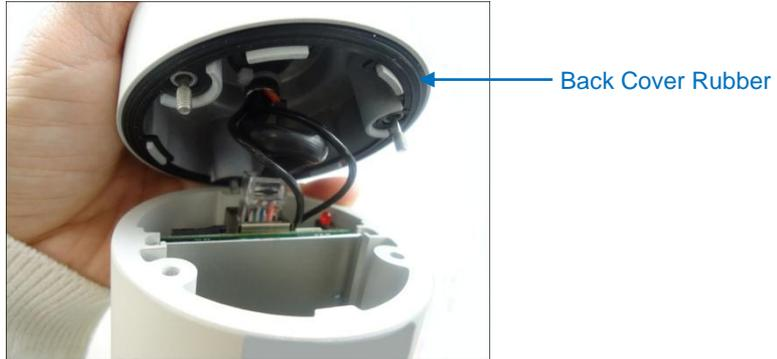
**NOTE:** Ensure that the rubber is properly aligned to the cover when closing the back cover.
