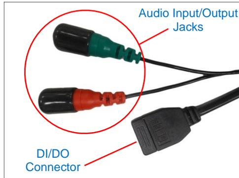
**NOTE:** If these connectors will not be used, leave the caps on to avoid water or dust from entering the connectors.
