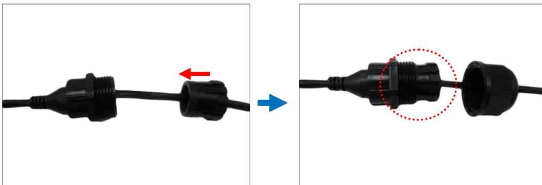
8. Attach the clamping nut to the cable gland body. Make sure the clamping nut is tightly secured and the sealing rubber is squeezed in to avoid water leakage.
