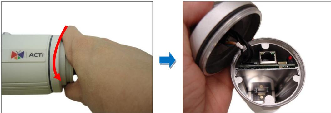
**NOTE:** Connectors are connected inside the camera, do not abruptly lift the cover.
