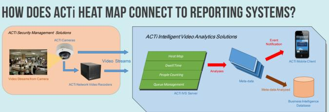
ACTi's heat map analyzes video streams from cameras or network video recorders to generate descriptive data information for each imaginary grid on the video. This data information, or meta-data, can be further processed and compared to trigger notifications to mobile devices if pre-defined conditions are met. Meta-data can also be saved and processed through analysis tools to provide demographical information, which can be used to further refine your subsequent business operation.
